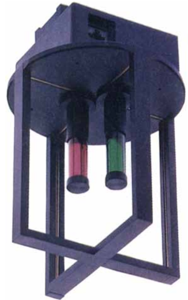
RADIO TRANSCEIVER links pads and other movable computer devices to the wired network. This unit, intended to be mounted on the ceiling, contains antennas in its crossed arms and two light-emitting diodes to signal its status.
