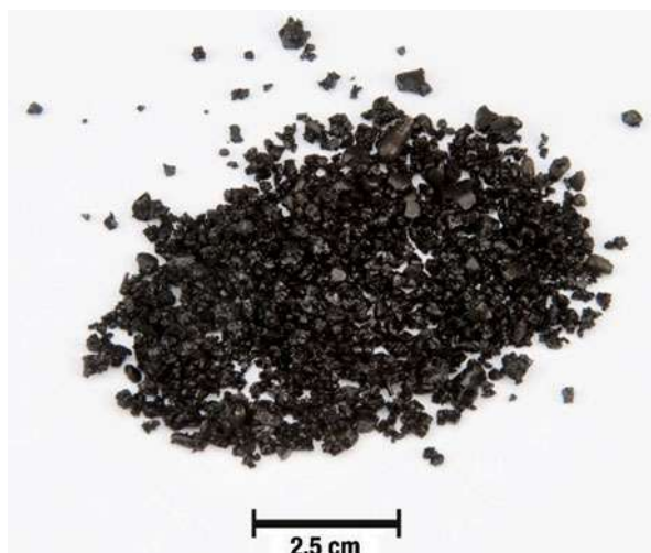
Fig. 30 Solid waste (mixture of ash, slag, and carbon char) removed from an entrained-flow slagging gasifier during operation
