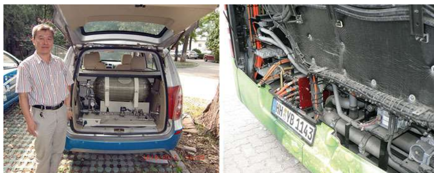
Fig. 65 Left: Standard car had the combustion engine converted into hydrogen by Professor Sun Baigang, BIT, Beijing, China. Right: The diesel engine of a Hamburg city bus is replaced by hydrogen fuel cells and storage (Preben Maegaard/Nordic Folkecenter for Renewable Energy)
