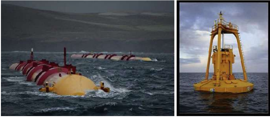
Fig. 9 Examples of oscillating body converters: Pelamis II ( left ) and PowerBuoy ( right ) (Courtesy of Pelamis Wave Power (2014) and Ocean Power Technologies Inc (2014))
