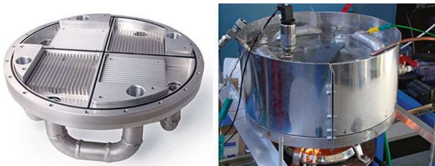
Fig. 10 The ambient temperature heat exchange plate of the cookstove generator developed by Aster is shown on the left-hand side , and the full machine is shown on the right being fired by a natural gas burner. A pot of water serves as the exhaust-side sink; the device is intended to provide hot water and electricity for citizens of developing countries (Photo by Kees de Blok, used with permission)
