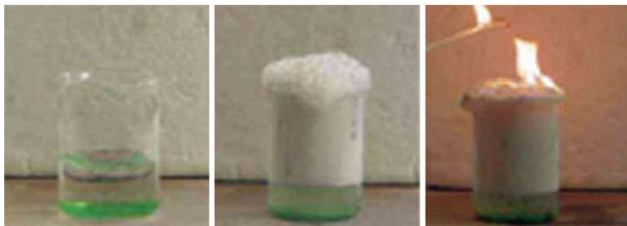
Fig. 11 Addition of calcium carbide to water (with some washing-up liquid added) and then ignition of the resulting foam
