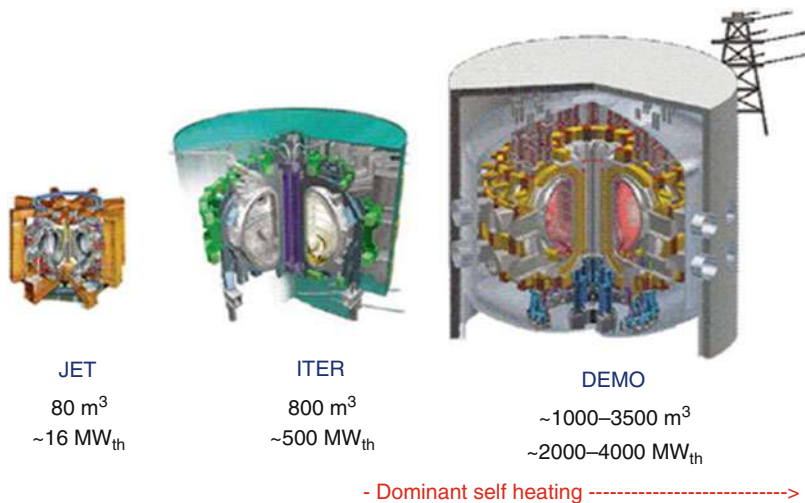
Fig. 25 The growth in scale of tokamak devices from JET, which produced the first DT fusion power, through ITER, aiming for Q = 10 at 500 MW thermal, to a DEMO reactor producing ~1GW electrical (Reproduction of Fig. 15 in Ikeda (2010))
