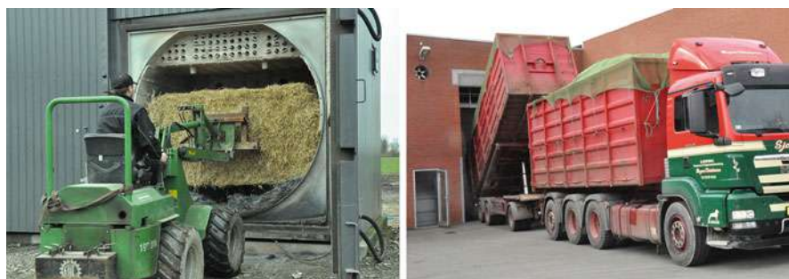
Fig. 19 Left: Boiler for central heating at farm for full-size straw bales. Right: wood chips are being unloaded at the central heating station (Jane Kruse/Nordic Folkecenter for Renewable Energy)
