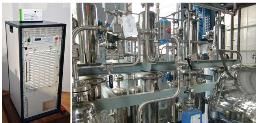
Fig. 61 H-TEC SYSREM PEM electrolyzer for decentralized production of hydrogen ( left ). A key technology for integration of wind, solar, and other renewable energies. ( right ) Pipe network for water, hydrogen, and oxygen of containerized H 2 package (Preben Maegaard/Nordic Folkecenter for Renewable Energy)
