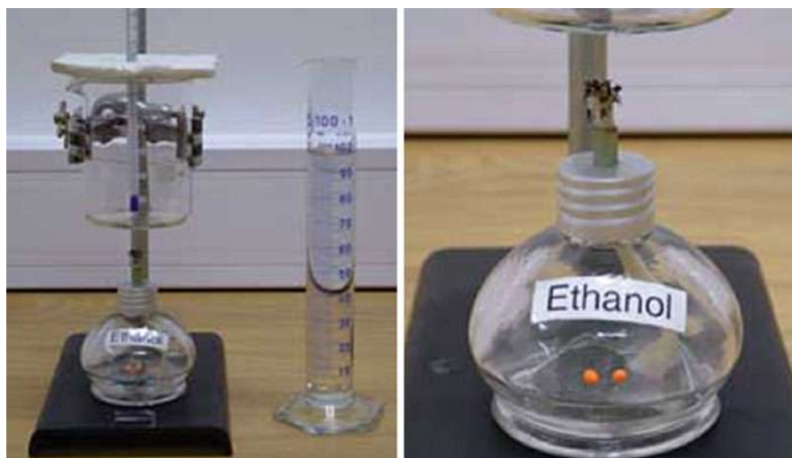
Fig. 15 Alcohol burner setup under a beaker to which a known volume of water is to be added
