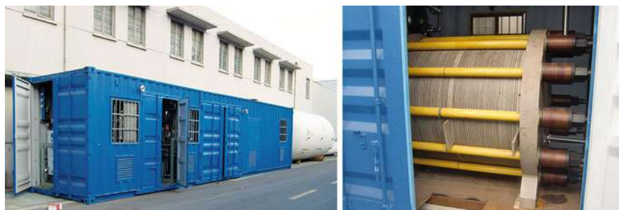
Fig. 62 Fully integrated 150 m 3 per hour hydrogen production package ( left ). Includes water treatment, power supply, electrolyzer, and ancillary equipment; ( right ) 150 m 3 per hour electrolyzer in container (Preben Maegaard/Nordic Folkecenter for Renewable Energy)
