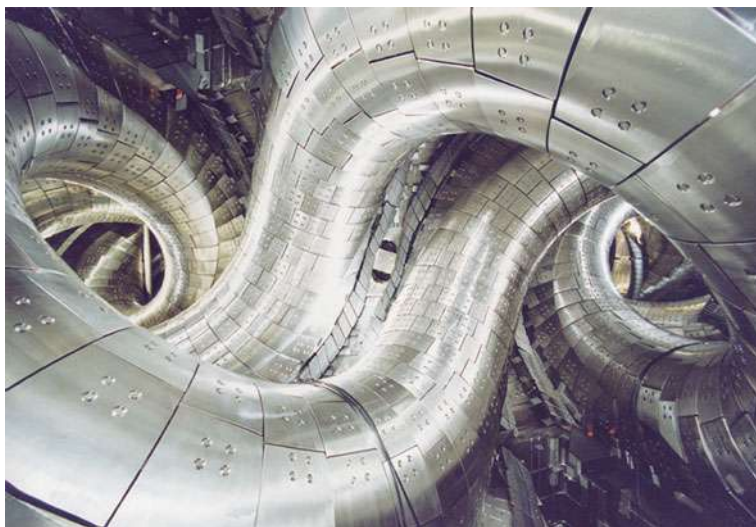
Fig. 24 Photograph of the plasma vacuum vessel of LHD : the Large Helical Device (Courtesy of the National Institute for Fusion Science, Japan). The major diameter of a twisted doughnut-shaped plasma is 7.8 m
