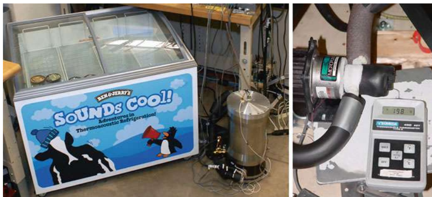
Fig. 7 A view of the regenerator-based thermoacoustic ice-cream storage cabinet built at Penn State University with sponsorship from Unilever/Ben & Jerry's. The thermoacoustic cooler is the silver unit to the right of the off-the-shelf storage cabinet. Heat was moved out of the storage cabinet and to the oscillating helium in the thermoacoustic machine by circulating ethanol within the copper tubing of the cabinet that typically carries R134a refrigerant and into the thermoacoustic machine's internal load heat exchanger. The photo on the right shows the pump that moved the ethanol covered with ice from condensed water-vapor in the air. A thermocouple reader shows the temperature of the ethanol to be -19.8^{\circ}\text{C} (Left photo by Greg Grieco, used with permission)
