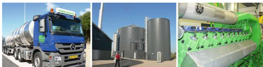
Fig. 51 Community biogas plant with CHP. The tanker truck ( left ) collects 400 t of liquid waste from farms daily. In the 7,000 m 3 Bigadan digester ( middle ), the biogas is produced which the Jenbacher gas engine ( right ) converts into heat and electricity (Jane Kruse/Nordic Folkecenter for Renewable Energy)
