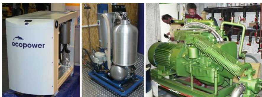
Fig. 37 Three types of small-size CHP. The Ecopower using natural gas ( left ), the Sunmachine wood pellet-fueled Stirling CHP, and small farm CHP using biogas (Preben Maegaard/Nordic Folkecenter for Renewable Energy)
