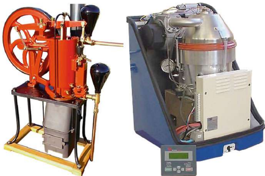
Fig. 11 On the left is photograph of a Rider-Ericson engine produced in the late 1800s and early 1900s. Notice the complicated linkage that connects the flywheel to the piston rods that penetrate the top of the piston cylinder. On the right is a modern Stirling machine made by Whisper Tech ( http://www.whispergen.com/ ) in 2002 that is used to generate electricity for residences, yachts, and motor-homes. Hidden in the stainless steel pressure vessel is a complicated linkage called a “wobble-yoke” ( left photo in the public domain, right photo credit: Whispergen)
