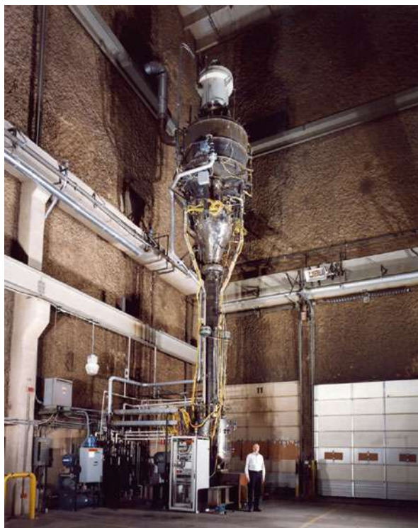
Fig. 9 A photo of the natural gas liquifier next to a six-foot (1.8 m) tall man shows the highest power thermoacoustic device ever built. At the top is a blower attached to the combustion chamber. The thermoacoustic engine is below the combustion chamber (the conical shaped component) and is connected via the wave tube to a vacuum can at the bottom next to John Wollan, one of the designers and builders of the machine. This device liquified 350 gal/day with a projected production efficiency of 70 % liquifaction and 30 % combustion of an incoming gas stream (Photo by Greg Swift, used with permission)
