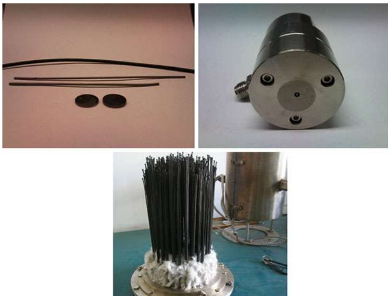
Fig. 7 (Top left) Typical sintered disk membrane (bottom), sintered hollow fiber (middle) and green hollow fiber (top), (top right) tube-in-orifice spinneret to synthesize hollow fiber and (bottom) hollow fiber membrane module consisting of 889 fibers
