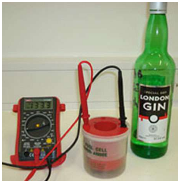
Fig. 16 Fuel cell using gin to generate electricity
