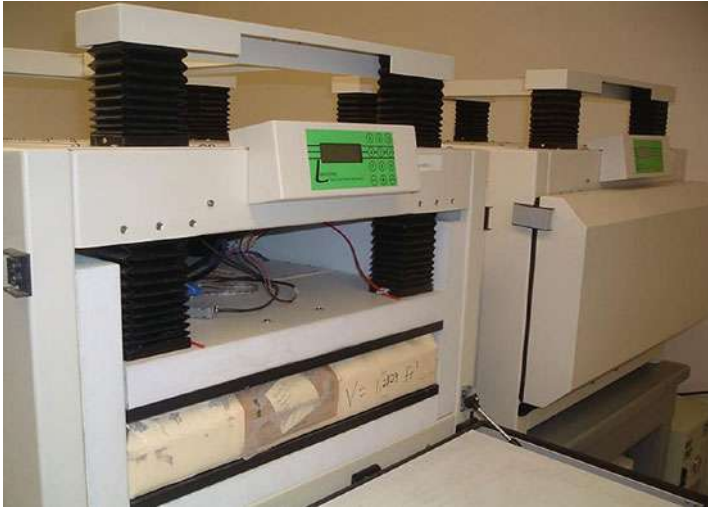
Fig. 1 Photograph of two heat flow meters ( open and closed ). The brown test specimen is between two black isothermal plates. The front is closed during a test
